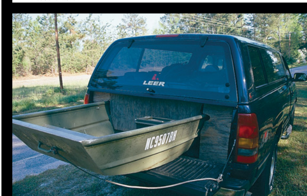
One of the best no-trailer fishing boats is the aluminum johnboat. It can be placed in the bed of a pickup or on the roof, and offers plenty of stability when handling fish over the side.
